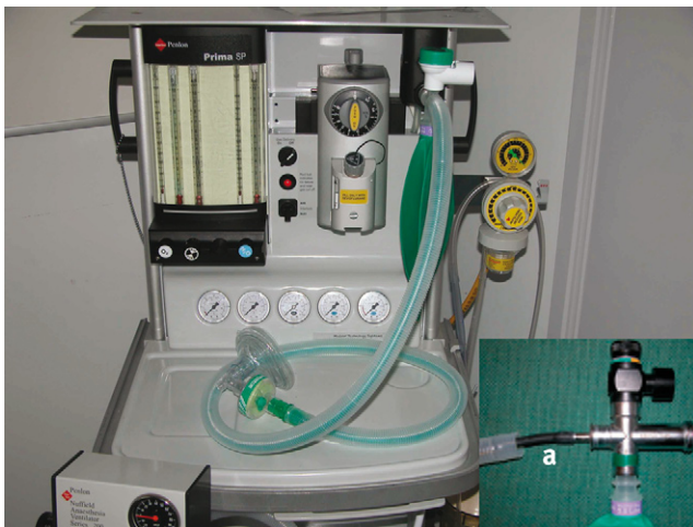
Figure 4 A coaxial Bain breathing system. Fresh gas is supplied to the patient end via the small inner tube. The inner tube connection (a) is shown in the inset figure.
